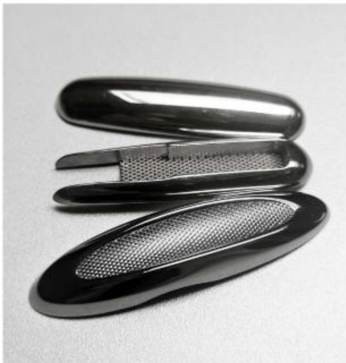
Fig. 9 Detail of textured MIM parts (Courtesy Gevorkyan)
