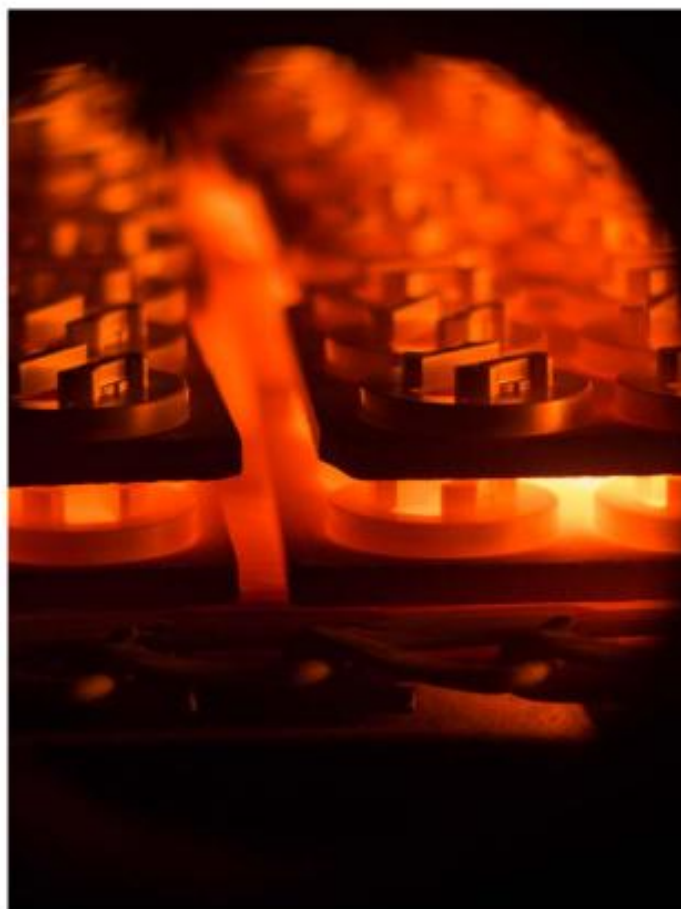
Fig. 3 Sintering of PM parts (Courtesy Gevorkyan)
